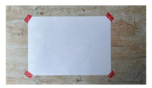
**Step 5:** Take your ruler, and draw a new line, starting from where the diameter line meets the bottom edge of the large circle, going through the middle point of the smaller circle, and finishing when you meet the edge of the large circle again.
