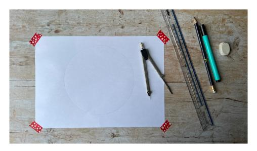
**Step 2:** Using the ruler as a guide, draw in the diameter of the circle with the pencil, i.e. a line from one edge of the circle to the other going right through the middle point.
