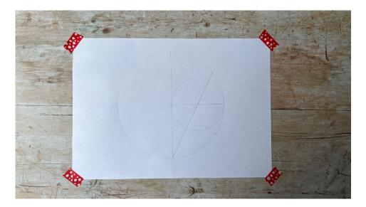
**Step 6:** Using the compass, place the point of the compass where the diameter line meets the bottom edge of the large circle. Set the compass to the width between that point and where the line you drew in Step 5 meets the near side of the smaller circle. Draw a semi-circle that cuts across the edges of the large circle on both sides.
